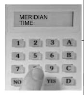
To part set Meridian go to the Keypad and key in your 4 digit PIN code and press 'B'.
